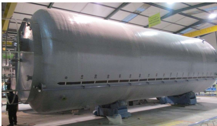
GRP SODIUM HYPOCHLORITE STORAGE TANKS
