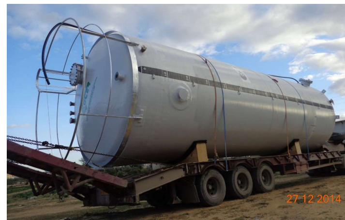
GRP HYDROCHLORIC ACID STORAGE TANK
