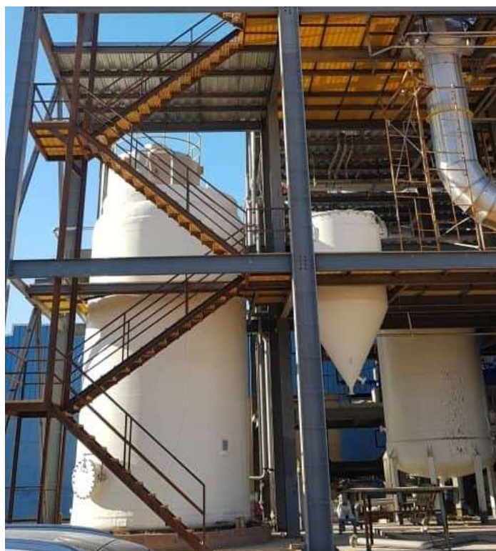
BRINE TANK , DECANter & SLURRY TANK
