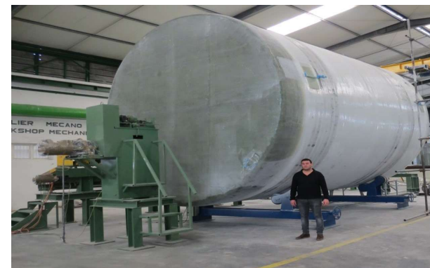
GRP FLUOROSILICIC ACID TANK
